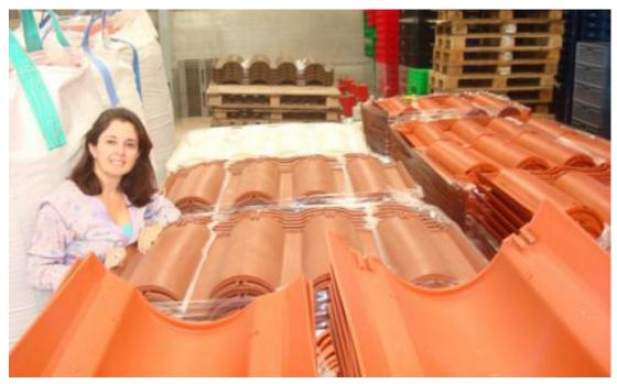
nanometric components which improve on the original properties of the raw materials. The shingles do not break, are not toxic, require no exposed screws and can resist hailstorms, it is claimed.
