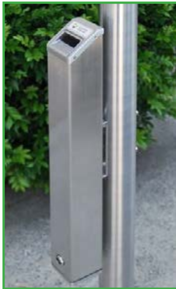
Pole-mounted receptacle secured with bolts vs. bands
