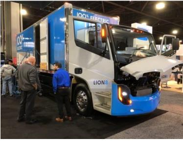
service on North American roads, recently unveiled an electric class 8 urban truck known as the Lion 8. It features up to 480 kWh of power, with an electric motor rated up to 350 kW, and a range of about 400 km. And it was drawing crowds on the trade show floor the night before. Lion's new class 8 all-electric truck was unveiled at TMC this week
